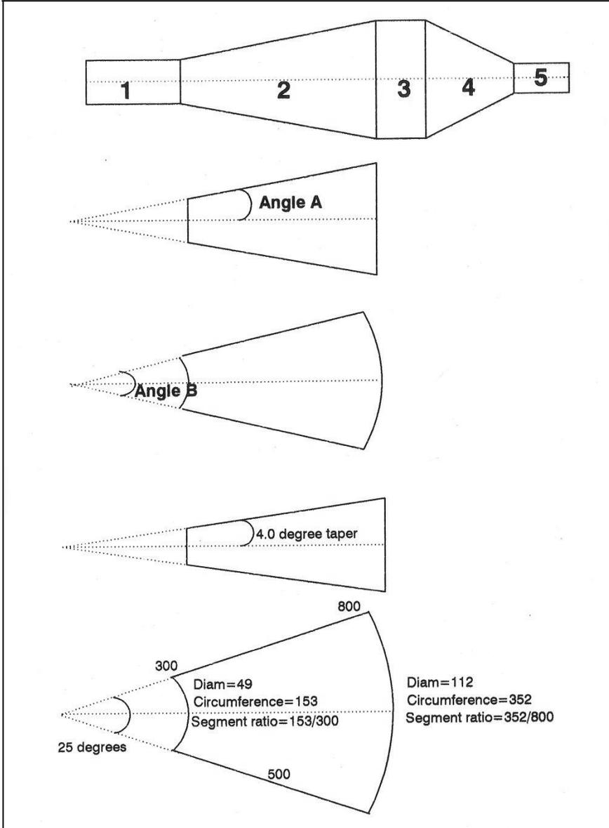
Figure 66 Exhaust cone development
