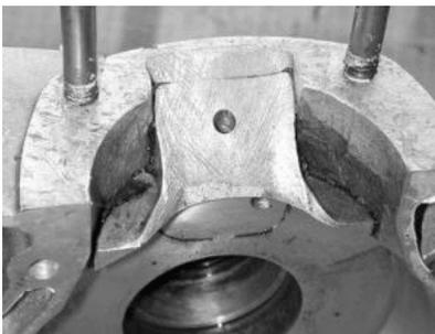
Figure 9 Crankcase stuffers
