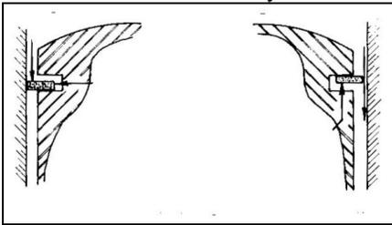
**Figure 21** Ring OK (left) and flutter (right)
