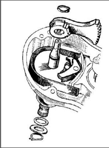
Figure 37 Post 1962 gear selector
