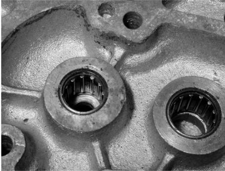
Figure 39 Gearbox with needle roller bearings
