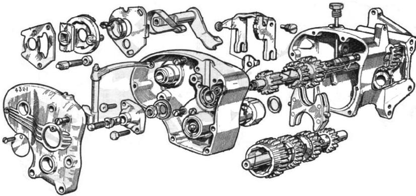
It is a straight-forward matter to pick a set of ratios that will do justice to the branch of the sport that we intend to pursue. As three and four speed boxes were used, it is best if we forget about the former as the combination of gears was less, and little is compatible between the two gearboxes.
