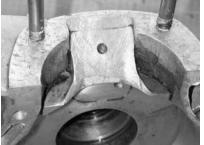
Figure 9 Crankcase stuffers
