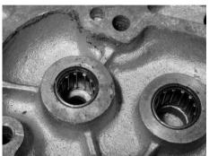
Figure 39 Gearbox with needle roller bearings
