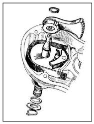
Figure 37 Post 1962 gear selector
